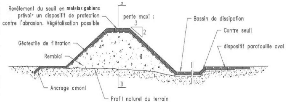
**SCH MA D'UNE DIGUE AVEC BASSIN DE DISSIPATION**
